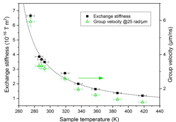
Fig. 1: Exchange stiffness and spin-wave group velocity in Gadolinium Iron Garnet as a function of temperature. Close to the compensation point, the exchange stiffness significantly exceeds the values obtained in metallic ferromagnets.
